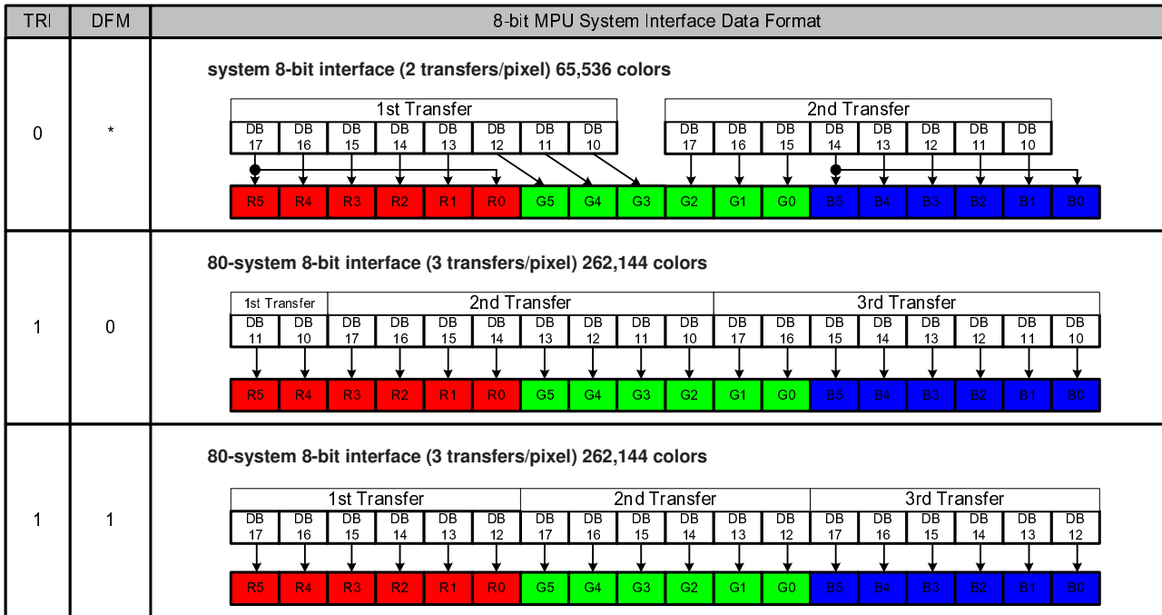
Figure5 8-bit System Interface Data Format
