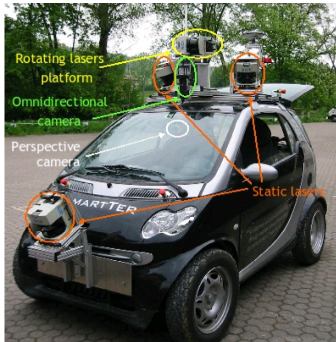
Figure 2.1: Side view of the SmartTer [1].
