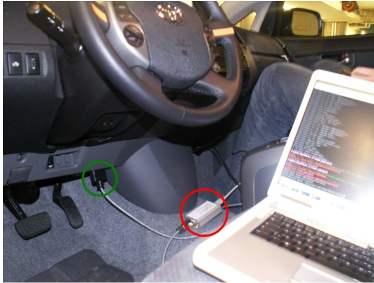
Figure 4.2: Connection between laptop and DLC3 port.
