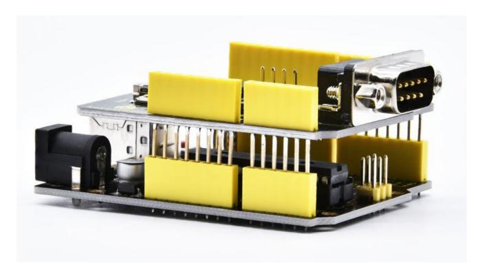
The shield provides a DB9 connector, so you can choose the interface according to your needs. It also comes with MicroSD card slot, so you can directly insert MicroSD card to store data.
